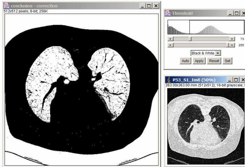
**Fig. 4.** GUI for teaching correct threshold value. Bottom-Right pane shows the original image. Left pane shows the affects of thresholding, which is controlled by the slider in the Top-Right.
