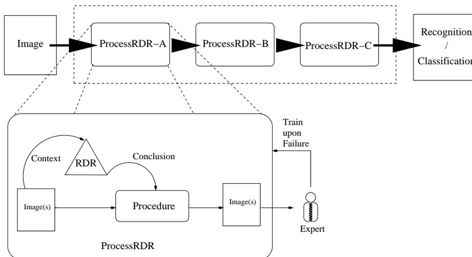
**Fig. 2.** ProcessRDR for a Computer Vision system.
